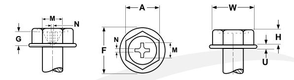
NOTE: Without any single set of standards for the size of cross-recess (Phillips) drives used in hex head machine screws, two sets of recess dimensions are listed below. Variations are due, in part, to differences in the tooling sold in the United States compared to that used by foreign manufacturers. Kanebridge offers this information as a service to fastener distributors and makes no recommendation re: which design is preferable.
